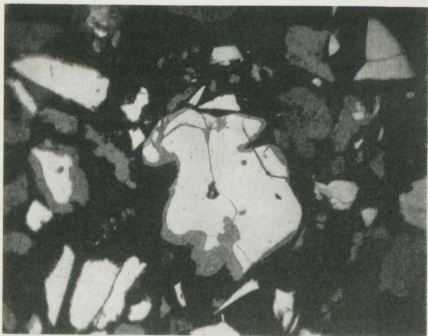
Figure 4a/b. Disseminated minerals in a porphyry copper deposit a) Covellite replacing chalcopyrite; b) Chalcocite coating or replacing pyrite. (Chuquicamata copper concentrate, 500 x, compare Amstutz , 1960, 61)
