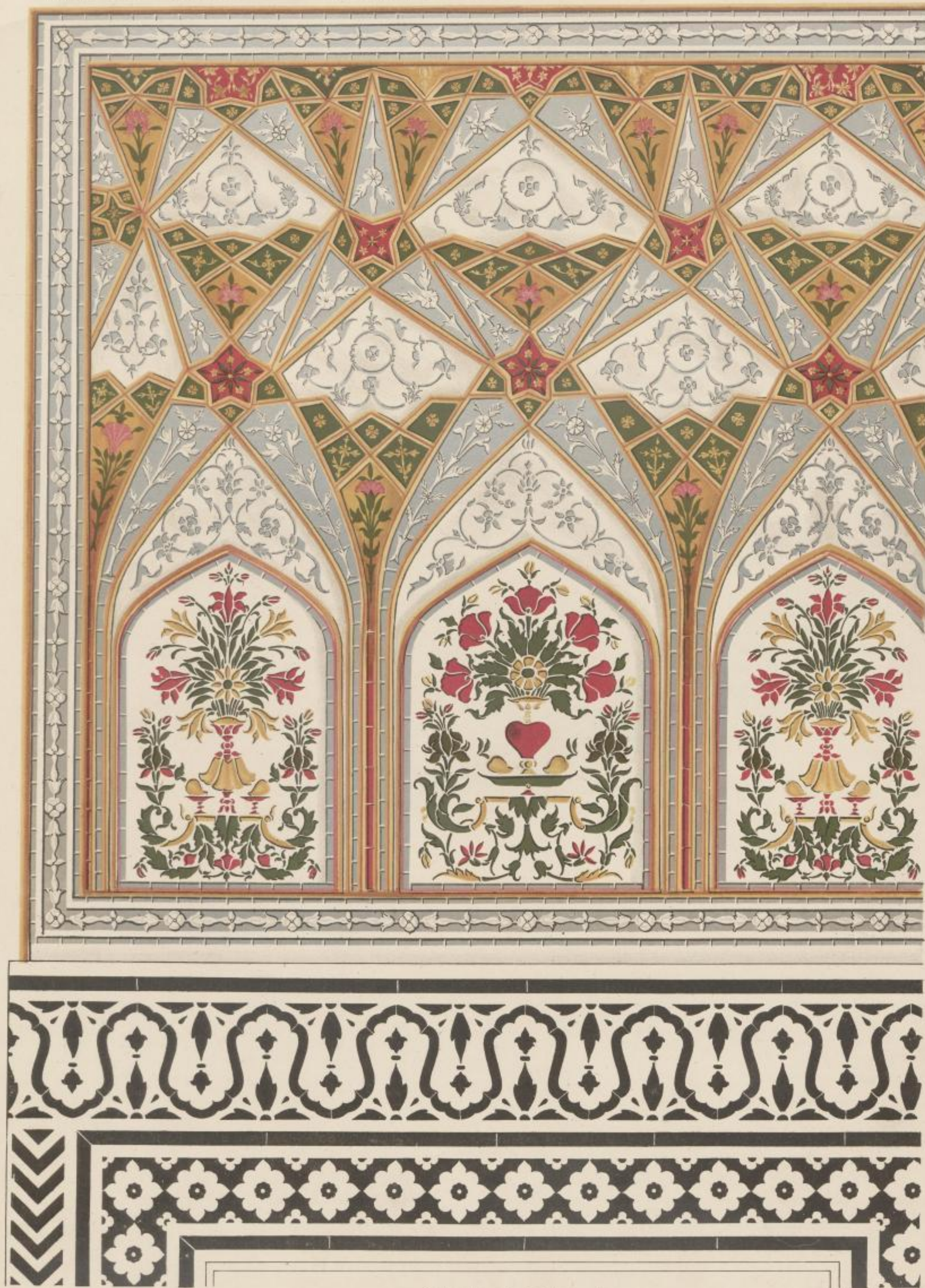
Surface decoration inside an archway. Tracery in plaster; coloured portions filled in with coloured glass, over concave copper reflecting shapes; the grey surfaces are glass mirrors set in plaster. Dado black and white marble polished.
