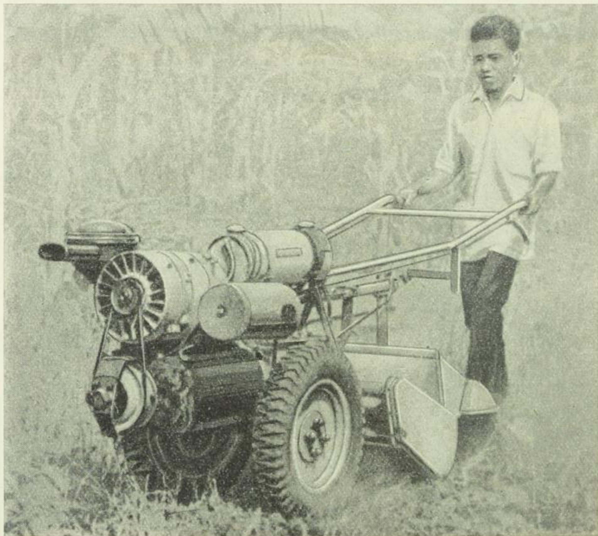
Fig. 6. Air-cooled two-wheel tractor
