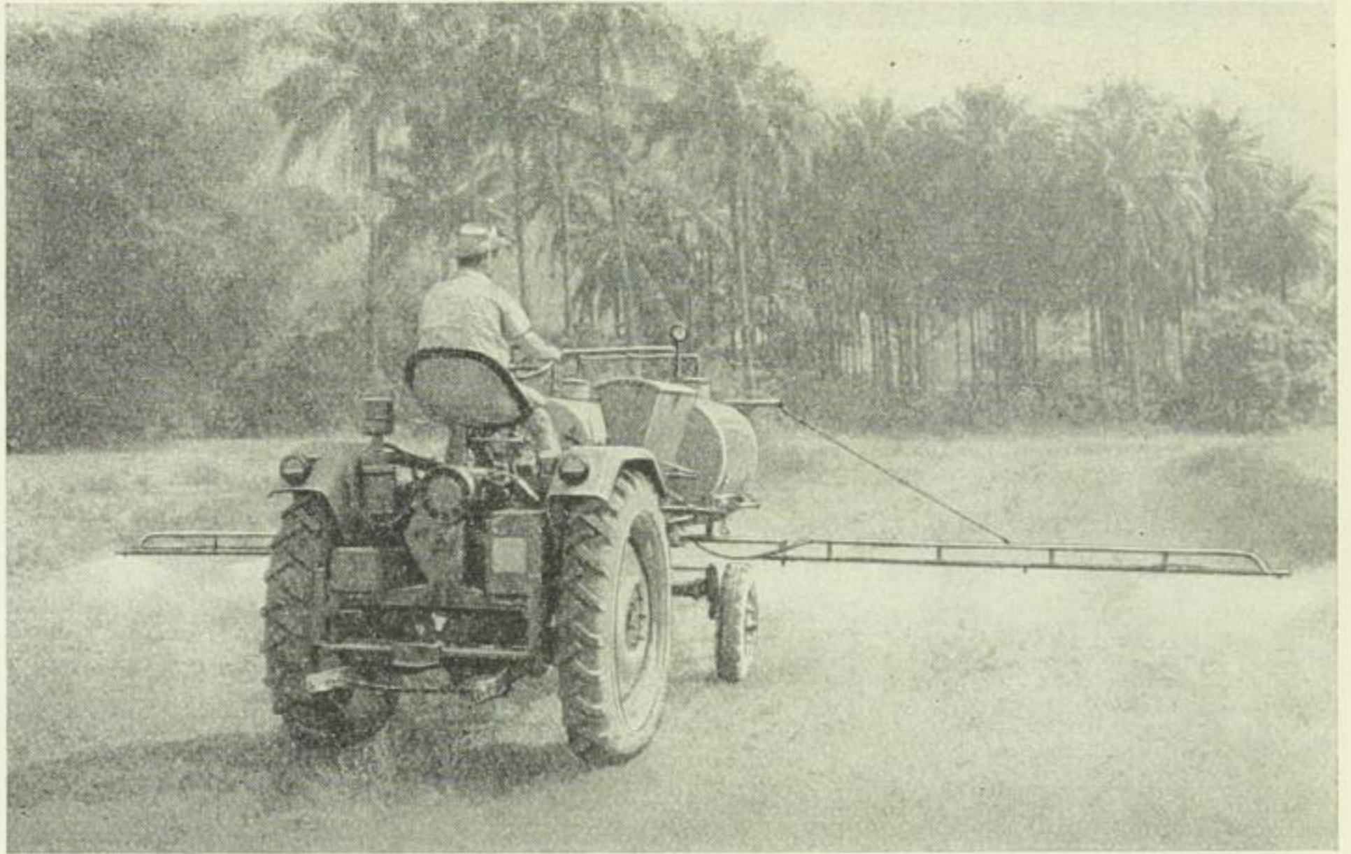
Fig. 9. Implement carrier with detachable implements for pest control (crop spraying) (Type: RS 09 / Photograph taken by the GDR delegation to Guinea 1960)
