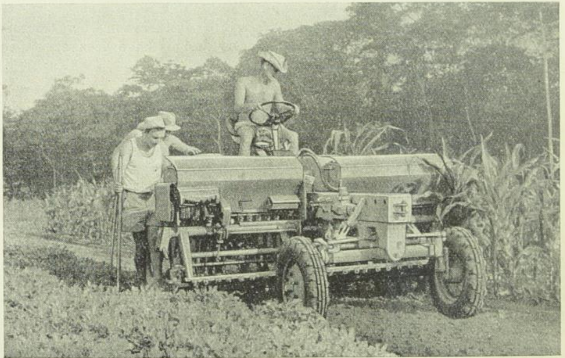
Fig. 10. Implement carrier with drilling machine (Type: RS 09 / Photograph taken by the GDR delegation to Ghana 1961)
