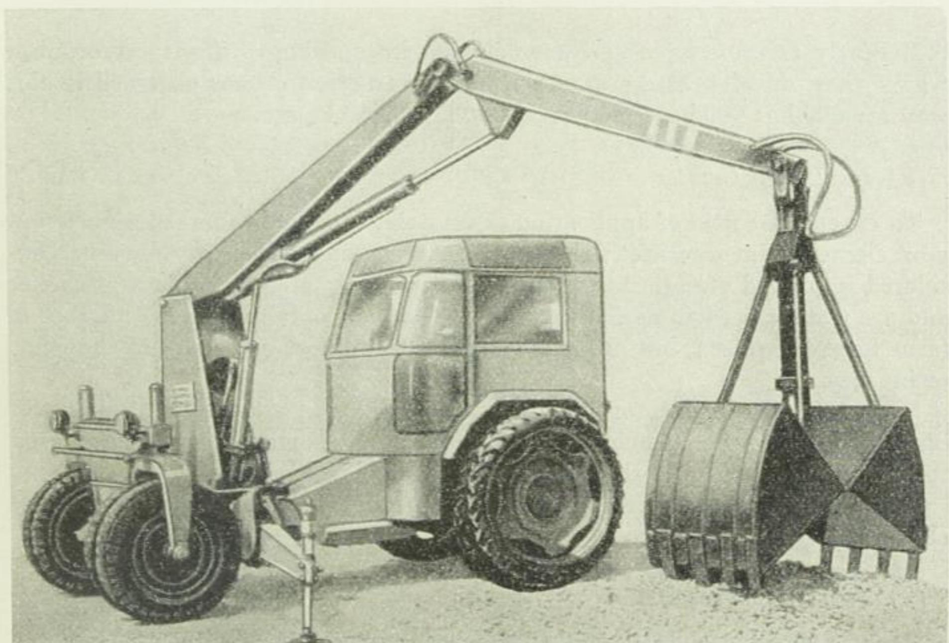
Fig. 12. Implement carrier with grab excavator; the swing jib crane is fully hydraulically operated (Type: RS 09)
