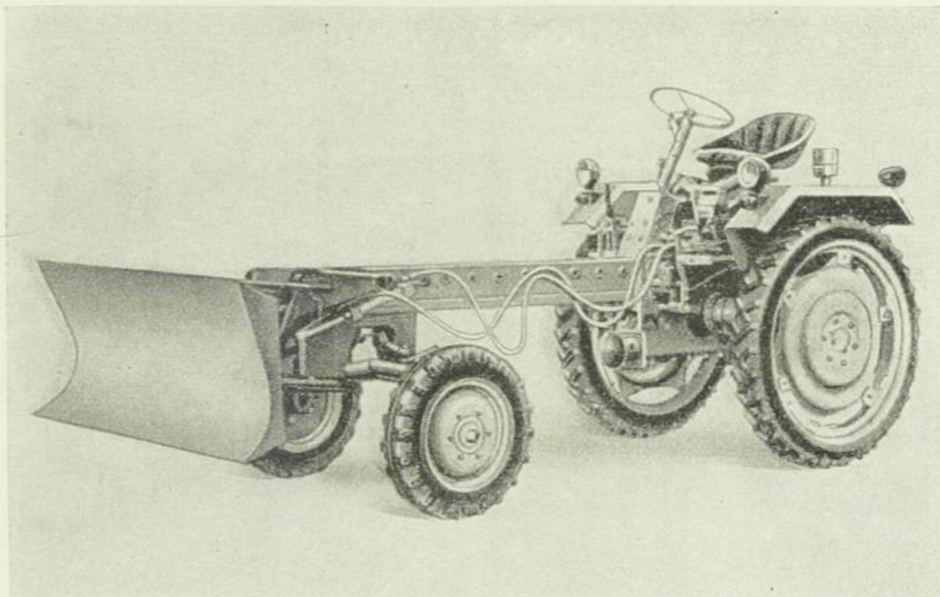
Fig. 11. Implement carrier with dozer blade
