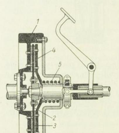
more complicated design. For example, several clutch springs can be arranged on the pressure plate or only one central spring be used (Fig. 198).
