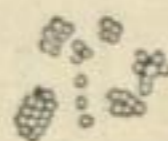
FIG. 5.—Same porcelain as Fig. 3. Granules isolated and in groups.
