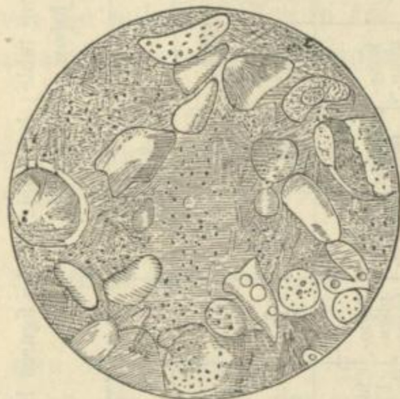
FIG. 2.—Part of a thin section of the bottom of a crucible of Berlin porcelain. \times 1500 .
