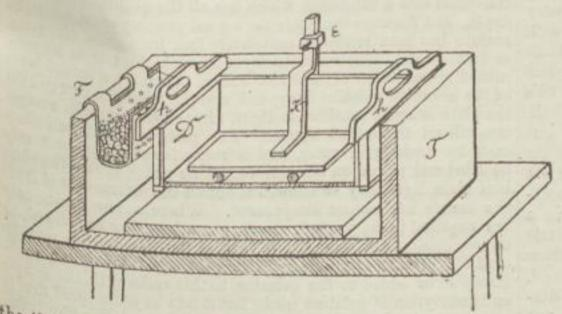
the Ordnance Survey Office at Vienna. The trough, T (see fig.), is a wooden box, lined inside with sheet-lead two millimetres thick, and coated with a suitable nonconducting compound. One very good mixture is the following :-
