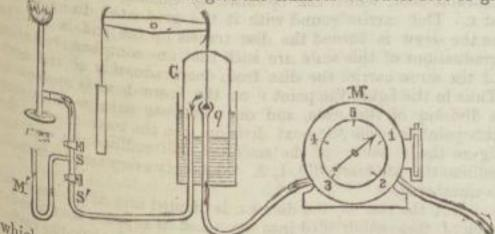
which pass through the meter in an hour. The gas enters at the middle through the meter in an hour. the middle of the back of the meter, and leaves it at the bottom, Passing thence to a governor, G, which consists of an inverted
