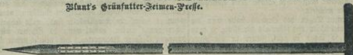
(Maximal-Thermometer zu Blunt's Patent-Press.)
